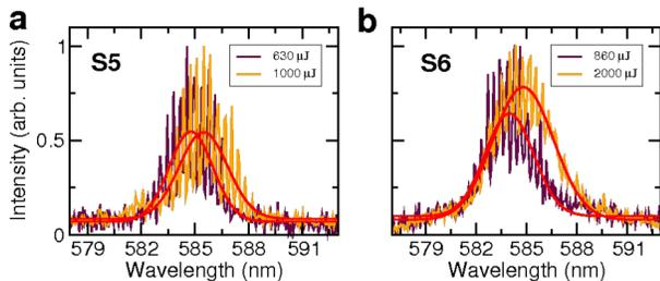
FIG. 4: **Kerr effect in the SPASER emission.** Experimental spectra from S5 (a) and S6 (b) taken at increased input energy. Solid lines are guides for the eye.
