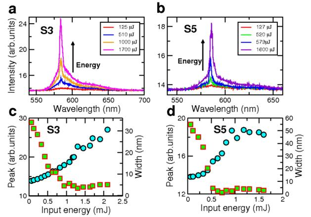
FIG. 2: **SPASER emission.** (a) Emission spectra at increasing pump energy of samples S3 and (b) S5; the insets show an enlargement of lowest energy spectra. (c) spectral width, calculated as half maximum full width (■) and height (●) for sample S3 when increasing input energy; (d) as in (c) for sample S5.
