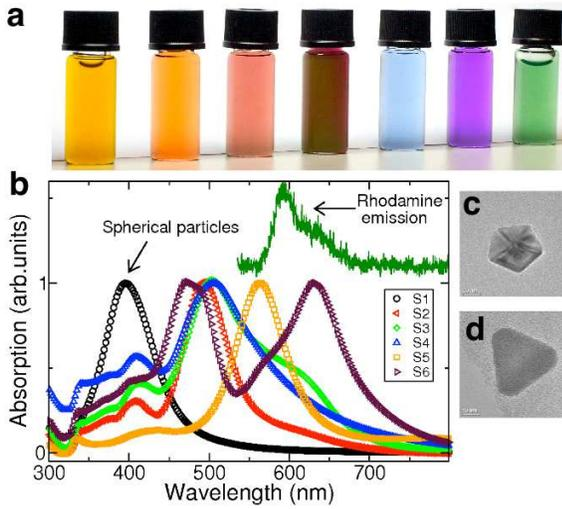
FIG. 1: **Morphology dependent colors.** (a) Pictures of selected samples; (b) Absorption spectra of various suspensions names S1-S6 and the emission of the adopted pure dye solution; (c,d) TEM images of silver nanodecahedrons and nanoprisms.
